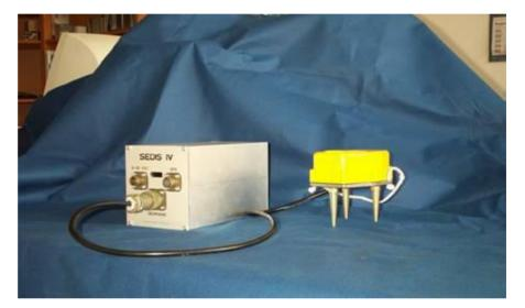
perfect tool to obtain accurate seismic data to evaluate reliable 2- and 3dimensional models of velocity distribution and reflectivities. Both marine and land versions record up to six channels (hydrophones and/or geophones) on hard disk with optional compression and choice of capacity - usually 10 GByte allowing up to 20 days of continuous data acquisition (see specification). A flash memory of 0.5 GByte is also built in the instrument.
