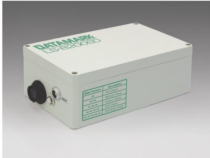
LS-8200SD is a single channel high-resolution data logger designed for large-scale crustal studies. Though small and low power consumption, the time calibration by GPS is also included. It is easy to use requiring a small team from preparation to the completion of the observation.
