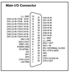
Note: Pins 9, 10, 26, and 27 have no connections on the DAS-1200 and DAS-1400.
