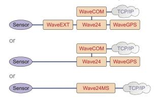
Communication computer WaveCOM can be used if data exchange is required. WaveCOM is connected to the Wave24 digital recorder, obtains data from it and provides them to other systems using TCP/IP based protocols. Whole configuration can be replaced by single mobile station Wave24MS, where all the modules are packed together in one case.
