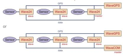
Communication interfaces of Wave24 make it possible to connect several recorders on a single line and share single WaveGPS time reference module. The data can be collected to one of the Wave24 recorders or to connected computer. This way, Wave24 can be a multichannel recorder or provide array features.
