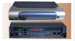
WaveCOM provides additional storage capacity to Wave24. Data can be recorded in SEED or GSE formats. WaveCOM supports both continuous and triggered recording modes.
