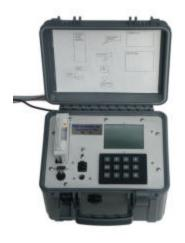
The PMD DR4000 is a *rugged*, *ultra low power*, *high-performance*, *versatile 24-bit resolution seismic recorder*. It is designed for the most demanding requirements in high performance seismic research.
