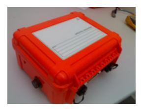
The eentec DR4050 is a *rugged*, *ultra low power*, *high-performance*, *versatile 24-bit and 18-bit resolution seismic recorder*. It is designed for the most demanding requirements in high performance seismic or strong motion research. Generally for structural monitoring and other seismic applications, only the 18-bit (low resolution 24-bit ADC) is required. The standard unit has an external sensor input.
