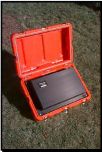
***Q730 system with the cover open. The sealed polyethylene enclosure, standard on all Quanterra products, is water tight.***
