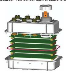
One or two removable disks reside in a sealed compartment that is accessed by opening a lid located on the top of the 130 case. The main electronics section is sealed with the lid open or closed.
