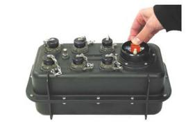
Data from the disk may be read on any PC/Workstation using a CF-II reader. Data can also be remotely downloaded from the 130-01 disk using FTP over LAN/WAN.
