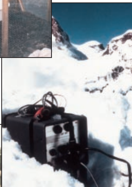
Twenty DASs like this recorder, were deployed on the Redoubt Volcano and surrounding glacier in Alaska. (1993-95)
