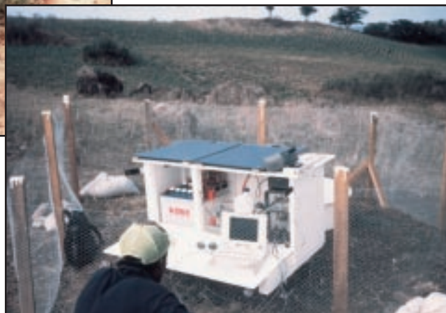
Twenty DASs like this recorder, were deployed on the Redoubt Volcano and surrounding glacier in Alaska. (1993-95)
