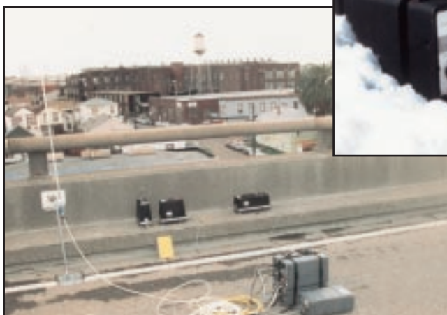
One of 25 aftershock deployments following the Loma-Prieta earthquake (1989). Equipment: Omega timekeeping, 72A-02 DAS, 72A-05 disk, 72A-04 power source, and 5 second velocity seismometers.
