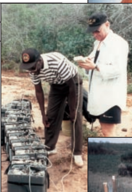
Being programmed prior to deployment, a group of REF TEK DASs are prepared for an active-source experiment in Tanzania, Africa. (1994-95)
