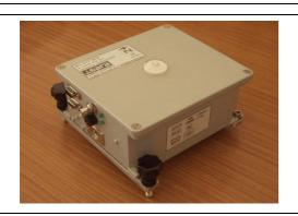
The SR97 is a low cost compact and rugged 16 bit digitizer. It allow to record seismic signal from sources giving +/-10V, or +/-5V. The unit is intended to be used for digitizing old analogic seismic radio-telemetered networks. Good noise results can be achieved using it with its preamplifier and antialias filter.
